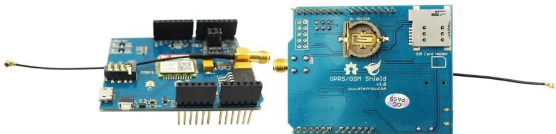
Figura 3-16 - SIM 800C GSM/GPRS Shield
