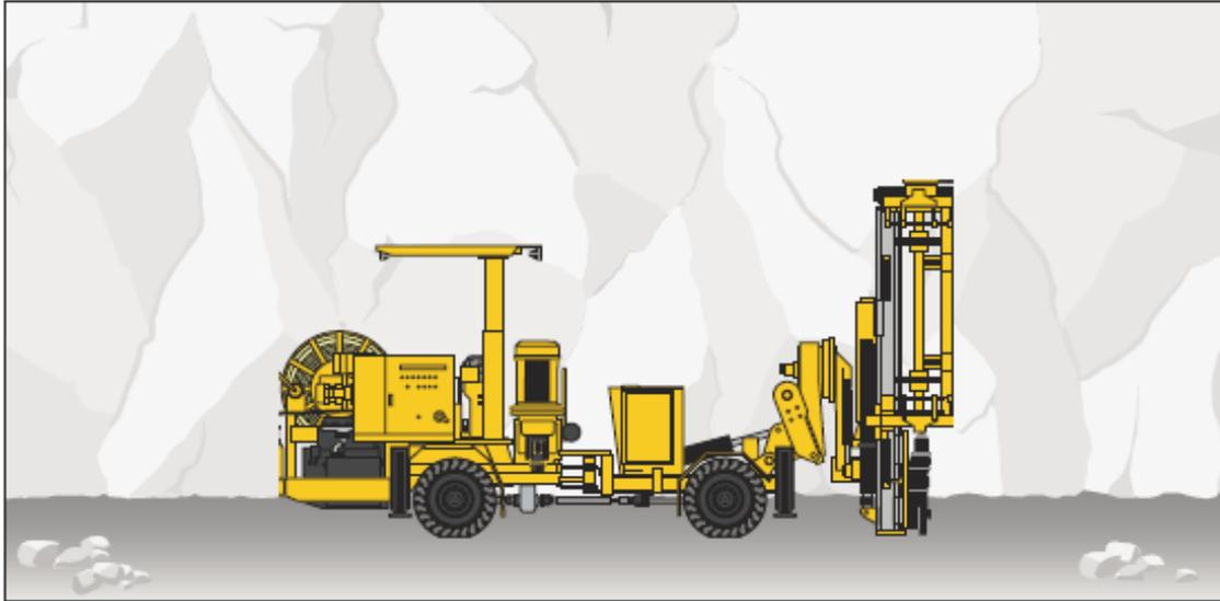
Production drilling rig adapted for small- to medium-sized drifts. Production drilling with topammer rock drill in the hole range 51–89 (102) mm. Different positioning configurations to match the method used.
