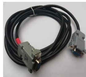
FIG. 53. CABLE RS232 (H/H).
